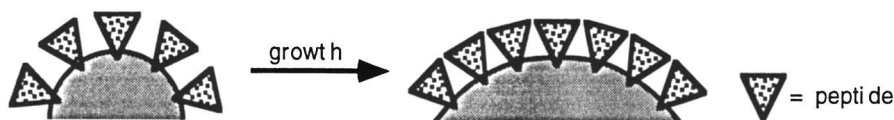
Figure 11. Diagrammatic representation of the growth of the CdS biomineral core, with surface coordination by phytochelatin peptides. As the core grows and the surface curvature decreases the peptides (which have fixed separations at the connection points on the core) are forced together and prevent further growth.
